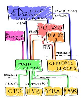
UC3A0/1 chips have quite a complex clock system as it can be seen from the figure. At start-up the UC3 runs at its internal RC oscillator that's 115 kHz. This means that the Main clock has been clocked from this RC oscillator and that the CPU frequency equals to 115 kHz. That's because by default the clock domain prescaler has been disabled. This also means that all the other clock domains, that are HSB, PBA and PBB, runs at 115 kHz frequency as well.
