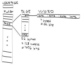
Flash Controller provides low-level access to the chip's internal flash memory, whose structure has been sketched in the figure above. The init function of the Flash Controller sets the flash wait state (zero or one, FLASH\_0WS or FLASH\_1WS, respectively). The last param of the init function enables/disables the sense amplifiers of flash controller.
