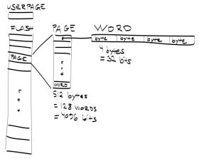
Flash Controller provides low-level access to the chip's internal flash memory, whose structure has been sketched in the figure above. The init function of the Flash Controller sets the flash wait state (zero or one, FLASH\_0WS or FLASH\_1WS, respectively). The last param of the init function enables/disables the sense amplifiers of flash controller.
