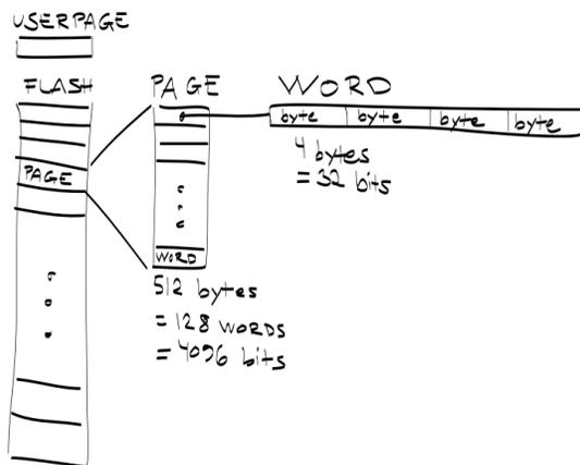
Flash Controller provides low-level access to the chip's internal flash memory, whose structure has been sketched in the figure above. The `init` function of the Flash Controller sets the flash wait state and the state of the sense amplifiers.
